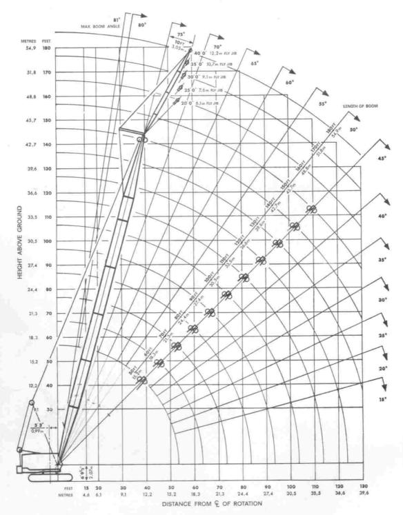
Maximum Allowable Boom and Fly Jib Lengths.
